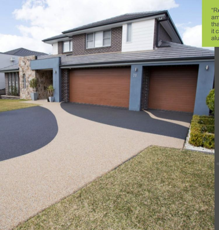
"Resin bound stone is unique amongst paving products in that, unlike segmental pavers, it can be shaped with the aid of aluminum edging."
